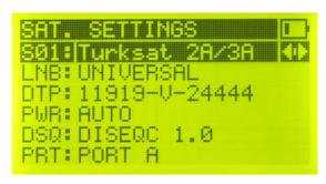
You can make the LNB and Diseqc adjustments of the satellites that are in the memory of the device. These adjustments will allow you to have quick access to commands in the other menus.
