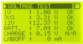
You may check all the supply values used during the o peration of your device, and there is a menu that makes it easier for you to contact the technical service in case of failu re of your device. You may follow the details regarding the maintenance or ca libration of your device on this screen as well.
